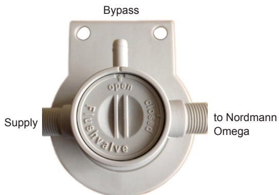
Fig. 18: Set valve to "Bypass" (flushing position)
